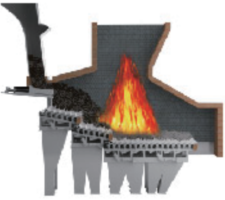
HPCC型炉排炉 (Hi-Pressure Combustion Control Stoker)
